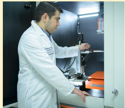
Dr. Jimenez inspecting a state-of-the-art biological irradiator that permits image-guided radiation therapy of small animals using built-in CT and bioluminescence imaging.
